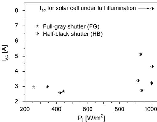
Fig. 5. The variations of short circuit current  $I_{sc}$  vs. light intensity  $P_i$  for solar cells under two kinds of shutters: FG and HB (a point for a fully illuminated solar cell is also reported).
