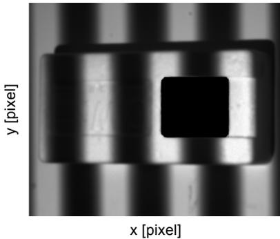
Fig. 8. The first pattern of the sinusoidal fringe.
