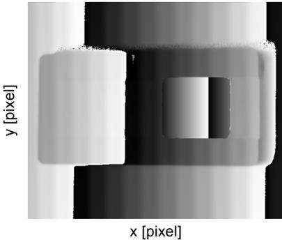
Fig. 11. The phase map obtained by Gdeisat's method.
