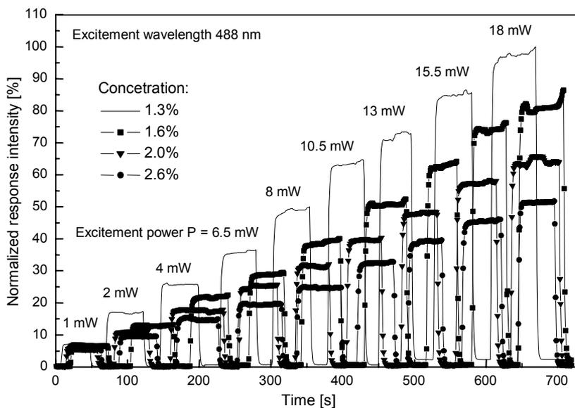
Fig. 4. Luminescence intensity for different dye concentrations and different laser exciting powers.
