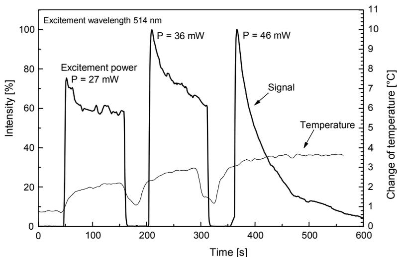
Fig. 3. Dye luminescence intensity characteristics in excitation power function.
