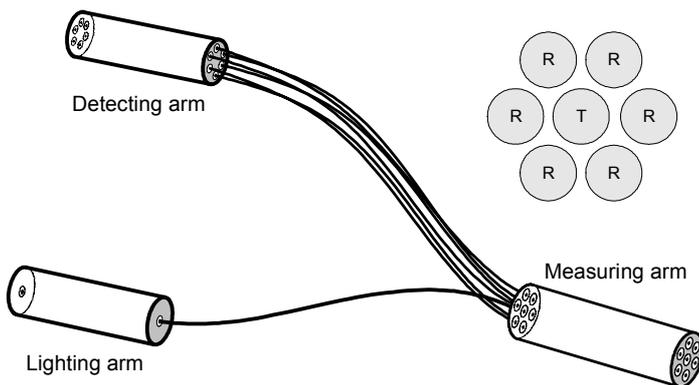
Fig. 1. Fiber sensor probe.
