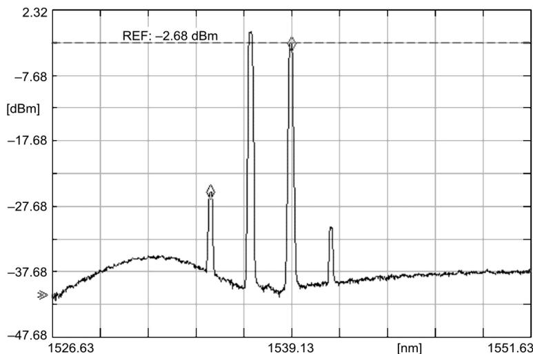
Fig. 2. Output optical spectra of wavelength conversion based on SOA. The wavelengths of the signal light, the pump light and the converted light are 1539.12, 1536.83 and 1534.68 nm, respectively.
