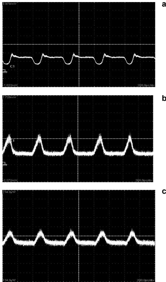
Fig. 3. Output waveform of the signal light (a), output waveform of the pump light (b) and output waveform of the converted signal light (c).
