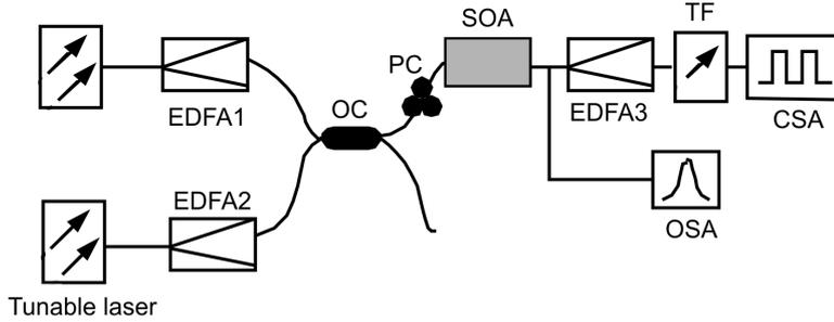
Fig. 1. Experimental setup for all-optical wavelength conversion based on SOA: TF – tunable filter, OC – optical coupler, PC – polarization controller, CSA – communication signal analyzer, OSA – optical spectrum analyzer.
