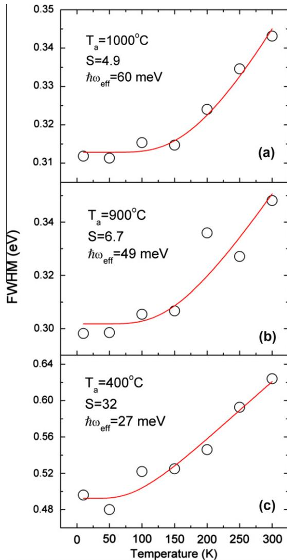
**Fig. 3.** FWHM of  $5d_{1LS}$  absorption band of  $Tb^{3+}$  ions calculated for samples annealed at (a) 1000, (b) 900 and (c) 400 °C. Fit to Huang–Rhys model has been also shown (solid line) together with the extracted parameters.
