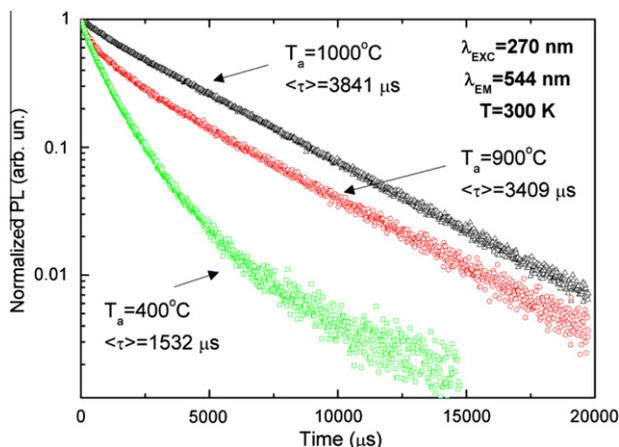
**Fig. 4.** Photoluminescence decay measured for  ${}^5D_4$ – ${}^7F_5$  transition. The excitation was through  $5d_{1LS}$  state.
