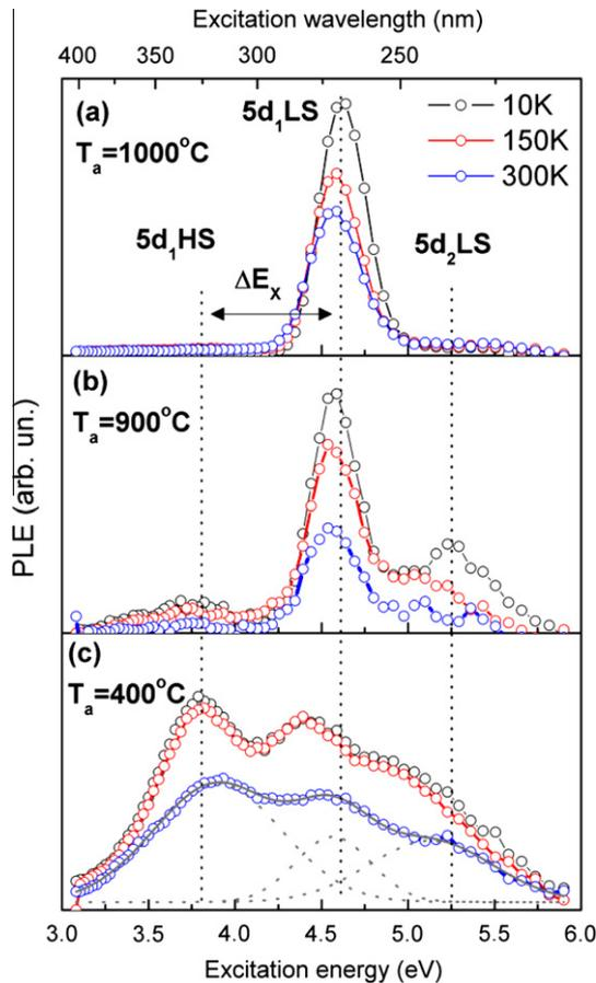
**Fig. 2.** Photoluminescence excitation measured as a function of temperature for samples annealed at (a) 1000, (b) 900 and (c) 400 °C. In the case of 400 °C sample, for 300 K, an exemplary fit with Gaussians is shown (also a slight offset from zero can be seen).
