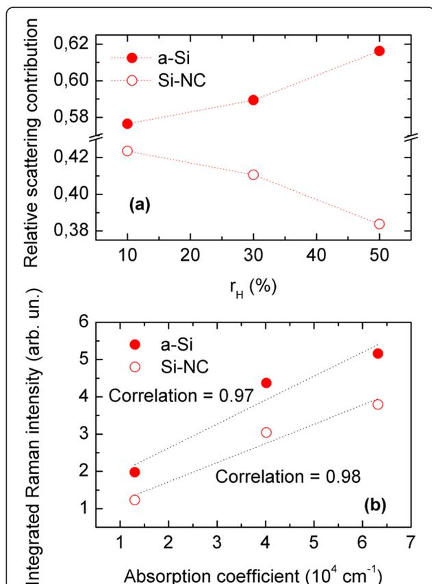
**Figure 2** Relative contribution of the HF (Si-NC) and LF (a-Si) Raman bands and their integrated Raman intensities. (a) Relative contribution of the HF (Si-NC) and LF (a-Si) Raman bands to the total scattering intensity is shown as a function of  $r_H$ . (b) Integrated Raman intensities of HF (Si-NC) and LF (a-Si) bands are shown as a function of absorption coefficient. Pearson's correlation coefficients have been also shown for a-Si and Si-NC.
