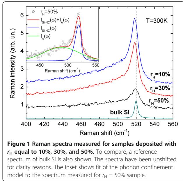
**Figure 1** Raman spectra measured for samples deposited with  $r_H$  equal to 10%, 30%, and 50%. To compare, a reference spectrum of bulk Si is also shown. The spectra have been upshifted for clarity reasons. The inset shows fit of the phonon confinement model to the spectrum measured for  $r_H = 50\%$  sample.
